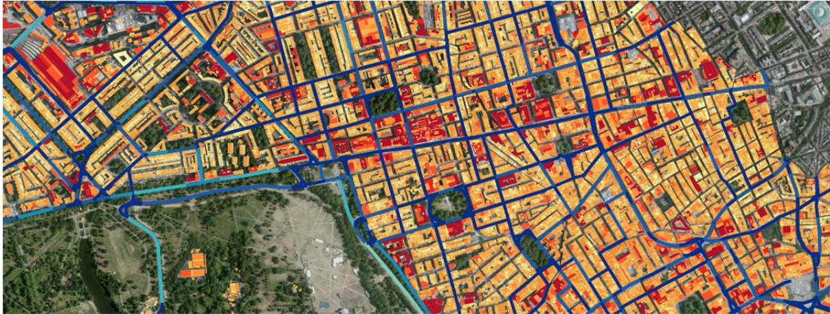
Annual energy intensity per building and per street calculated for the City of Westminster, London
